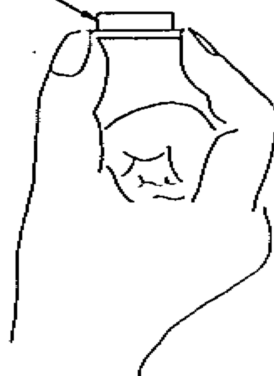
Fig. 9.6 Disconnecting the FPC Cable Connector
